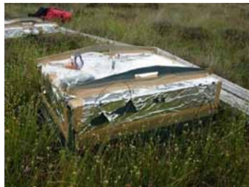
Figure 2.2. Static chamber employed to measure CH 4 and N 2 O fluxes.
