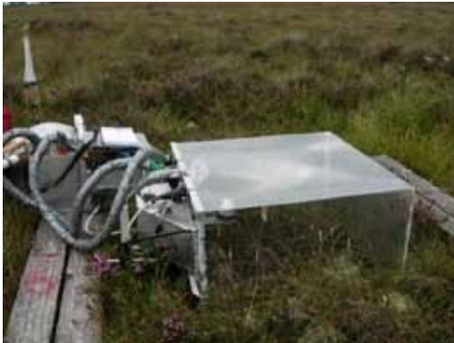
Figure 2.1. Static chamber employed to measure net ecosystem exchange (NEE).
